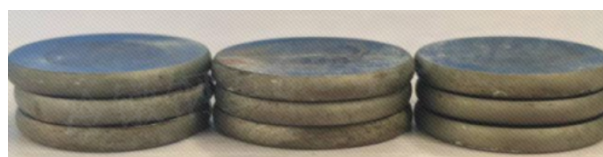
图2 盐浴态 \phi 7 mm规格QM1020盘条1/6冷顶锻 Fig. 2 1/6 Cold upsetting of \phi 7 mm QM1020 wire rod in salt bath state
